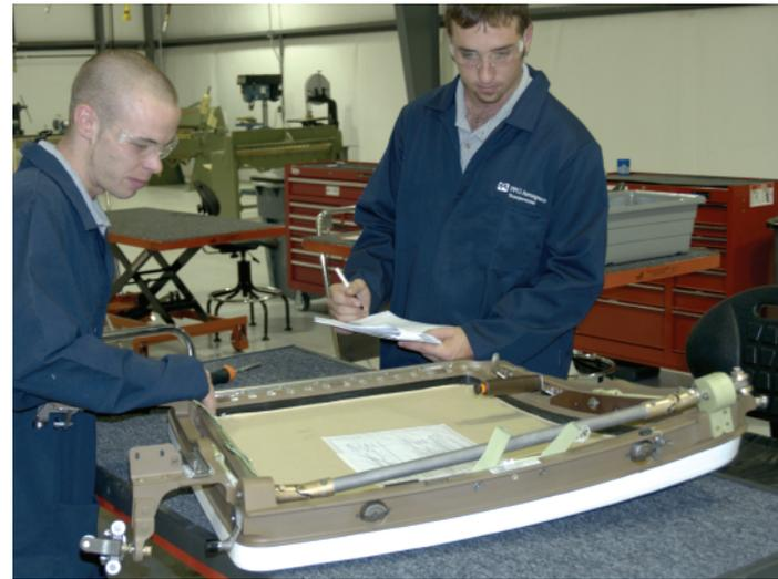
**Above:** Certified technicians inspect an overhauled Boeing 777 No. 2 framed window assembly.
