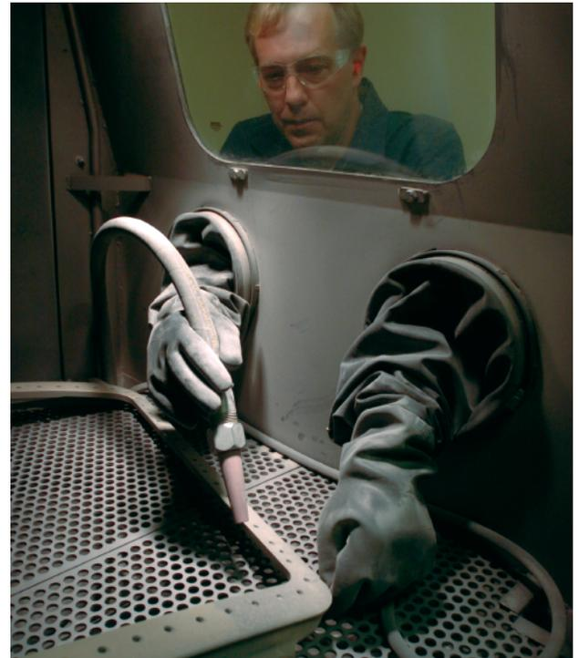
*Parts are cleaned using a blast media system that removes organic material while protective coatings remain.*
