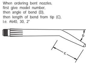
When ordering bent nozzles, first give model number, then angle of bend (D), then length of bend from tip (C), i.e. #640, 30, 2"
